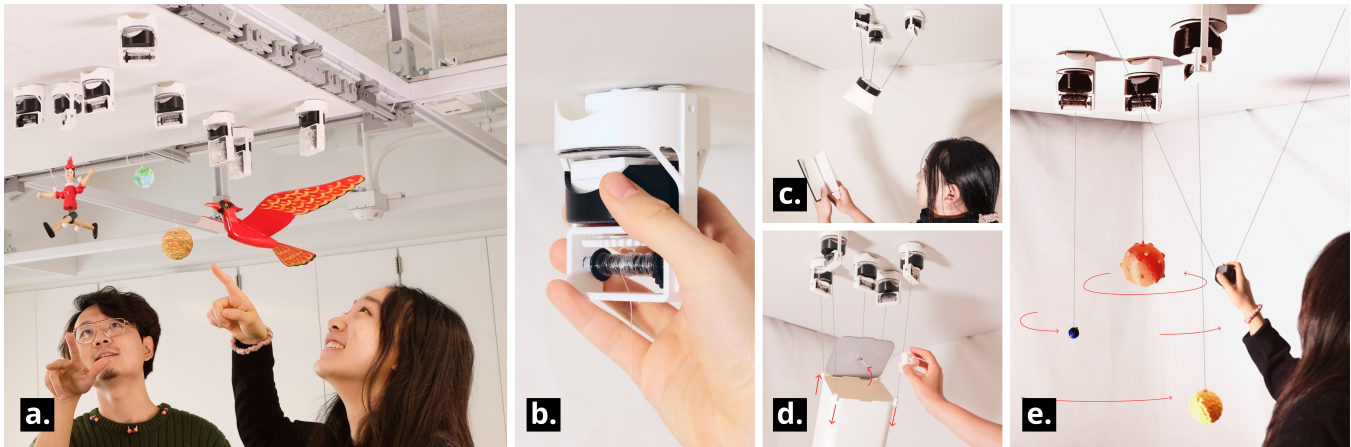
Figure 1: AeroRigUI: (a) users are tangibly interacting with everyday objects, controlled in the air by (b) RigBots – self-propelled swarm robots with a reeling mechanism. AeroRigUI provides controllability of objects and deployability in everyday spaces, allowing for applications such as (c) dynamic lighting, (d) tiltable storage container, and (e) interactive astral representation.
